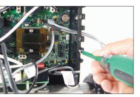
Insert the plastic holder and 2 screws back in place. Make sure the 2 cable wires are secure in place.
