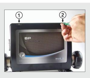
Use a phillips screwdriver to remove the 2 top screws that hold the system cover in place.
