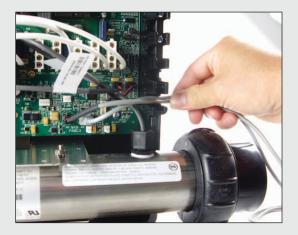
Place the Wi-Fi cable and Control Panel cable inside the wire holder.
