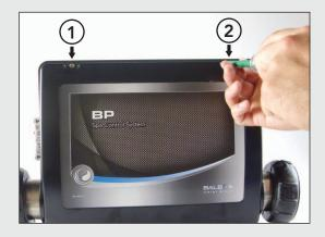
Use a phillips screwdriver to remove the 2 top screws that hold the system cover in place.
